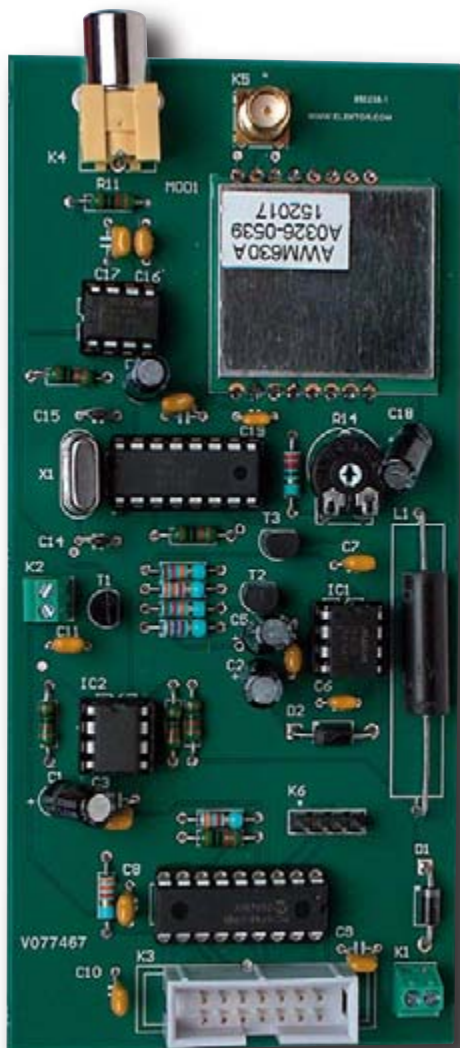
Figura 5. Components mounted on two of our prototype boards. Above: transmitter; below: receiver.
